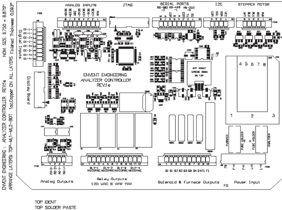
**Figure 2: Controller Board Layout & Power Input**
