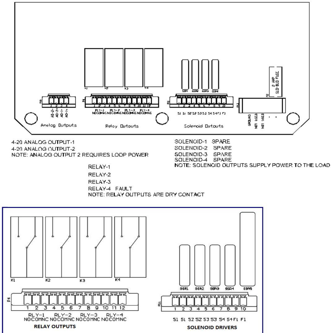
Figure 5: Relay Outputs & Solenoid Drivers
