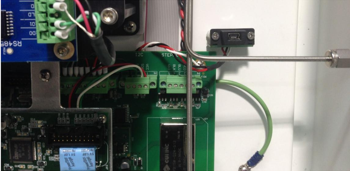
**Figure 3: TFS-2/TFS-YP USB Communication Connection**
