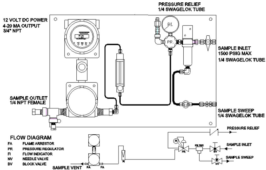
Figure E-5: M70XP standard sample system drawing
