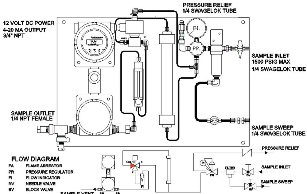
Figure E-7: M70XP standard sample system with auto-zero drawing
