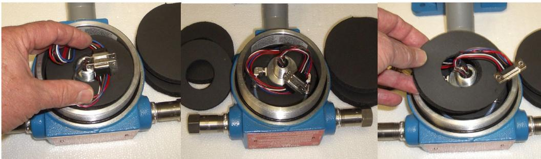
**Figure G-14: Sensor replacement procedure**
