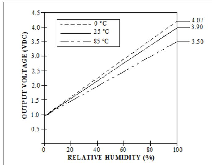
Figure C-3: Output voltage vs. relative humidity at different temperatures
