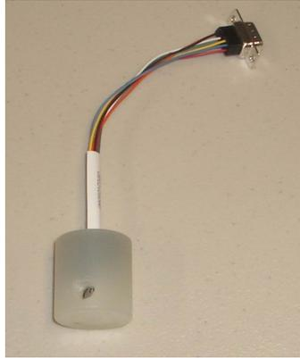
**Figure C-1: Polypropylene moisture sensor**
