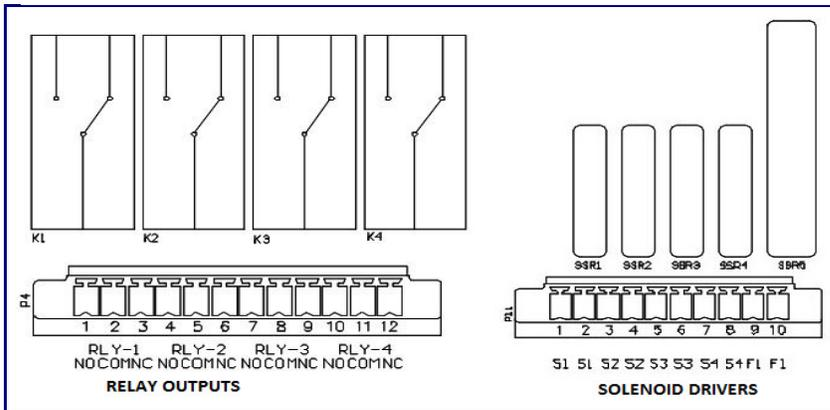
Figure 5: Relay Outputs & Solenoid Drivers
