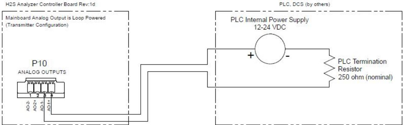
PLC Set for Externally Supplied Loop Power (Three-wire Transmitter)
