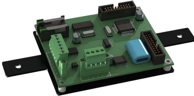
**Figure 21: Ethernet Communication Card**
