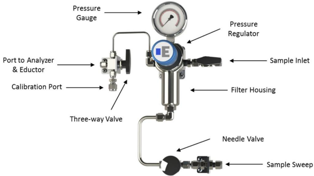
**Figure 17: Alternative Standard Sample System**
