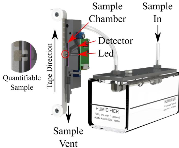
**Figure 1: H<sub>2</sub>S Analyzer Principle of Operation**
