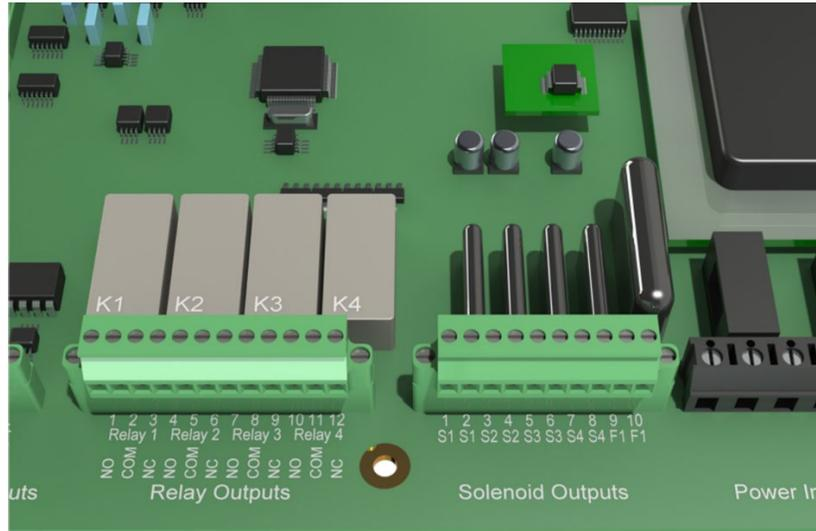
**Figure 6: Relay and Solenoid Outputs**
