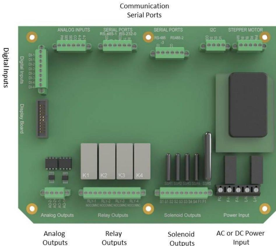
**Figure 5: Controller Board**
