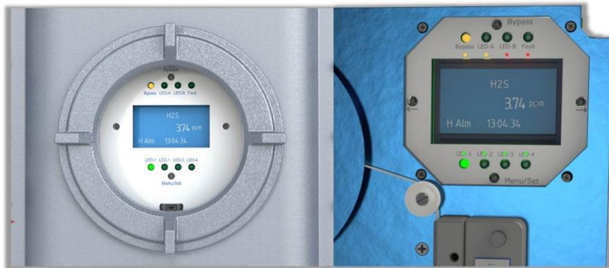
**Figure 22: 330S Display (left) & 331S Display (right)**
