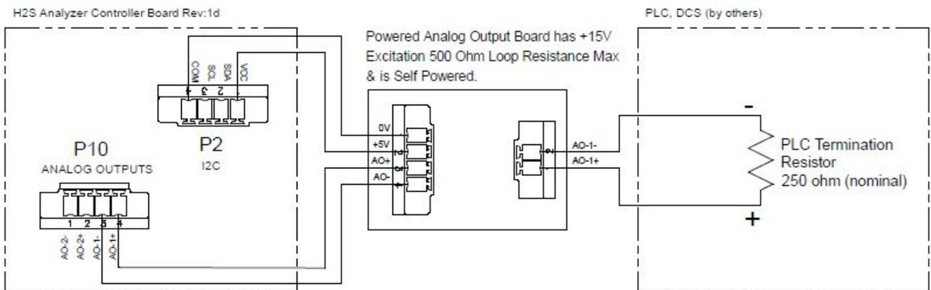
Figure 7: AO 4-20 mA Output Wiring Options
