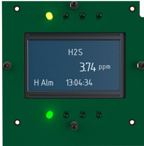
Figure 9: 330S & 331S H<sub>2</sub>S Analyzer Graphic Display
