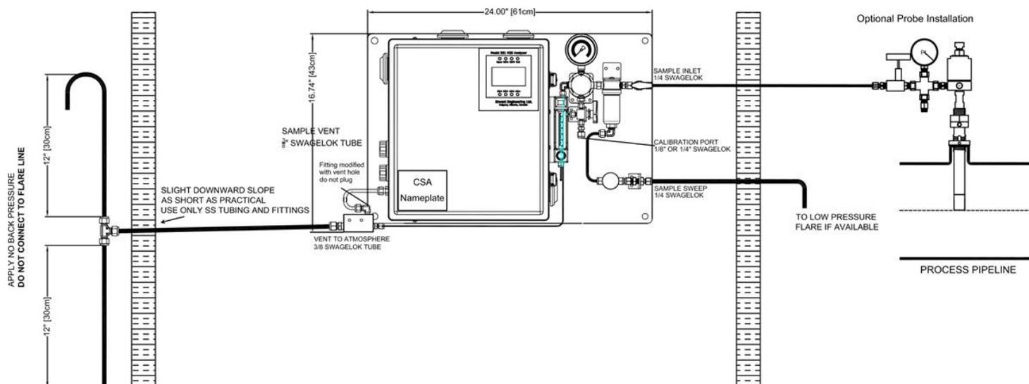
**Figure 4: Recommended Venting for 331S (Same for 330S model)**
