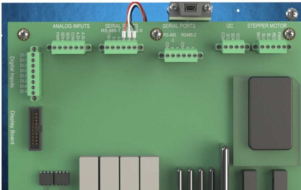
**Figure 8: RS-232 Serial Port wired to a Mini-USB Female Connector**
