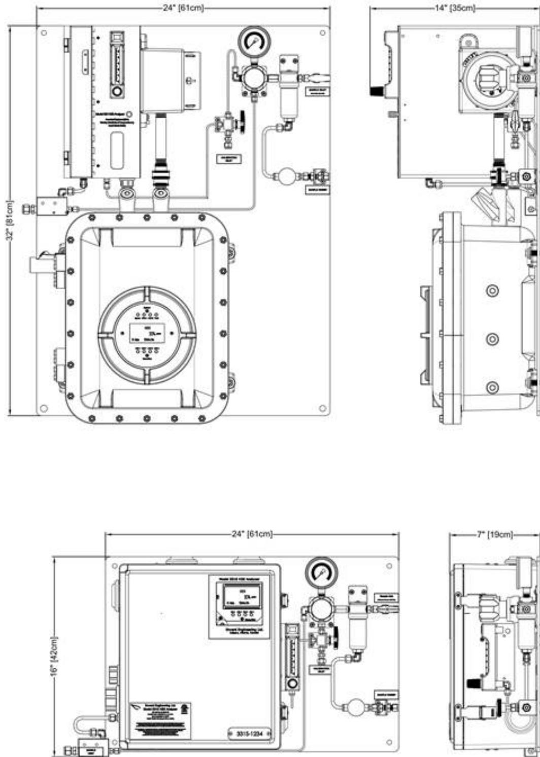
Figure 3: Space Requirements for the 330S & 331S H2S Analyzers
