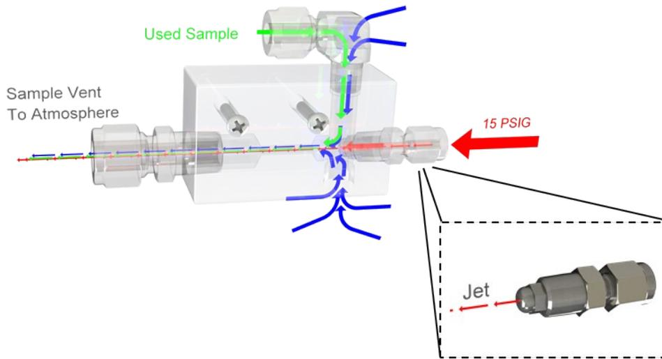
Figure 14: Eductor Block (Venturi Effect)
