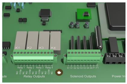
Figure 6: Relay and Solenoid Outputs
