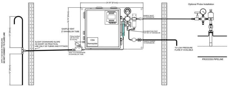
Figure 4: Recommended Venting for 331S (Same for 330S model)
