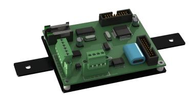
Figure 21: Ethernet Communication Card
