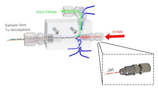
Figure 14: Eductor Block (Venturi Effect)
