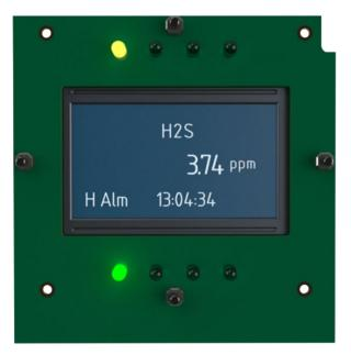
Figure 9: 330S & 331S H2S Analyzer Graphic Display
