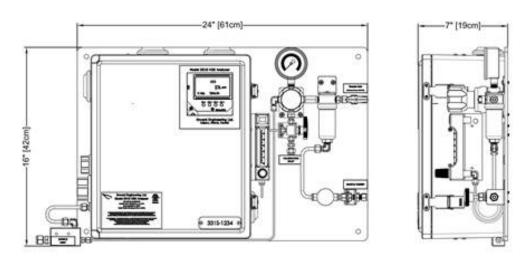
Figure 3: Space Requirements for the 330S & 331S H2S Analyzers
