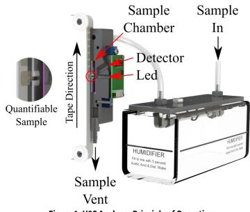
Figure 1: H2S Analyzer Principle of Operation
