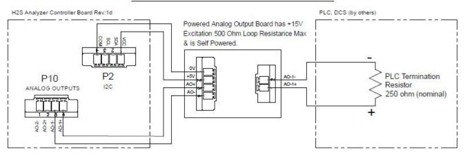
Figure 7: AO 4-20 mA Output Wiring Options
