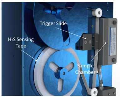
Figure 11: Trigger Slide Installed on a 330S H2S Analyzer (Applicable for 331S Analyzers)
