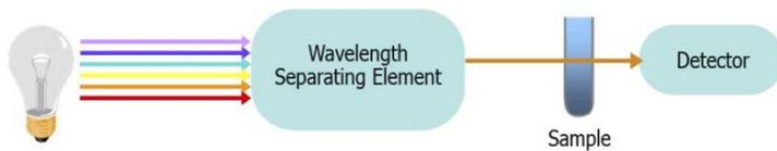
The TFS analyzers use an advanced spectral decomposition algorithm. The resulting spectrum is called the absorption spectrum, which acts as "fingerprints" used to identify the sample components and/or quantify the composition of the sample.
