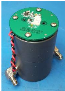
Figure 11: Assembled ppm O 2 sensor.
