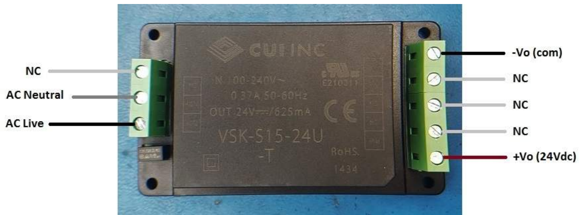
Figure 13: CUI inc VSK-S15-24U-T Switching Mode Power Supply (NC=no connection)
