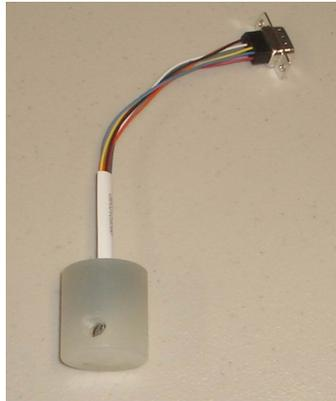
**Figure C-1: Polypropylene moisture sensor**
