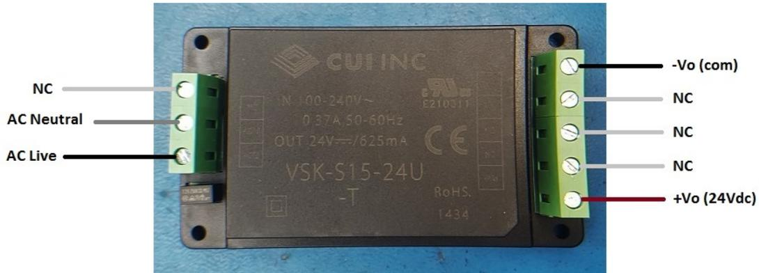
Figure APPENDIX D-15: CUI inc VSK-S15-24U-T Switch Mode Power Supply
