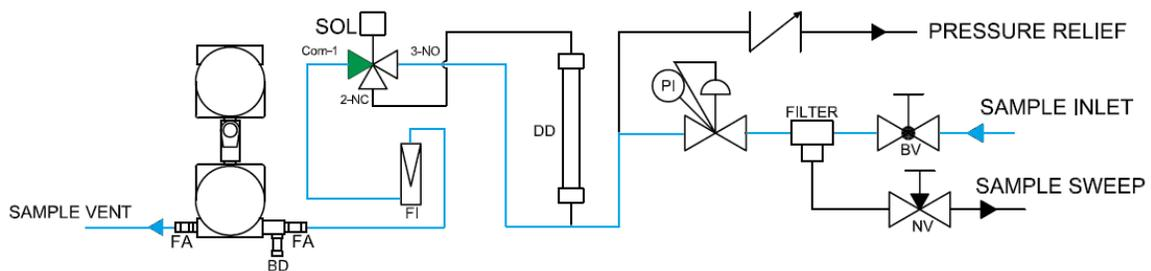
**Figure F-10: Sample system flow diagram in Run mode**
