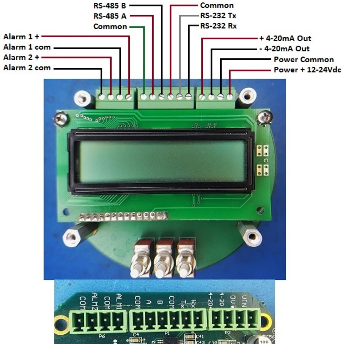
Figure E-8: Customer connections
