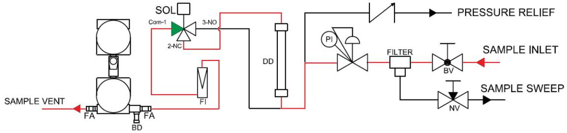
**Figure F-11: Sample system flow diagram in auto-zero mode**
