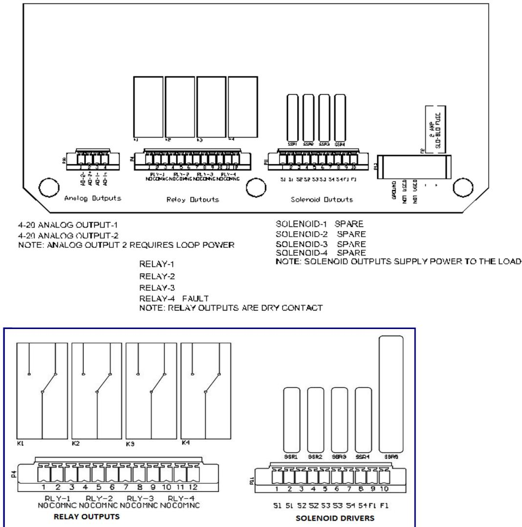
Figure 5: Relay Outputs & Solenoid Drivers
