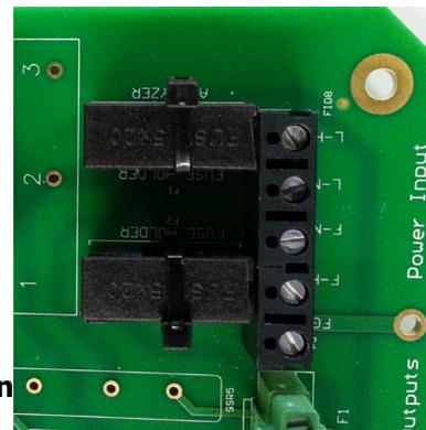
**Figure 7: Fuse Installation**
